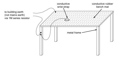
Figure 1.1 Typical Anti-static Bench Set-up
